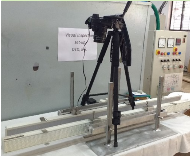
(L) the visual inspection setup (R) Visual Inspection of small scale (~50mm length) W monoblock mock-up after HHF test showing various surface defects such as pinholes, craters of melted zone and re-solidified metal droplets, and cracks.
