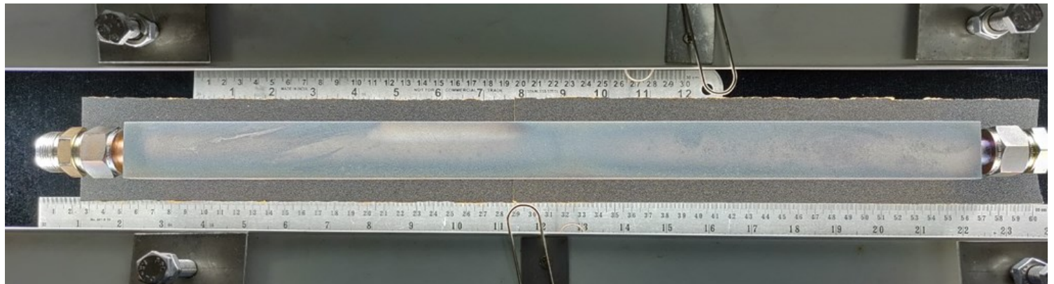
Visual Inspection of medium scale (~480mm length) W coated CuCrZr mock-up after HHF test.
