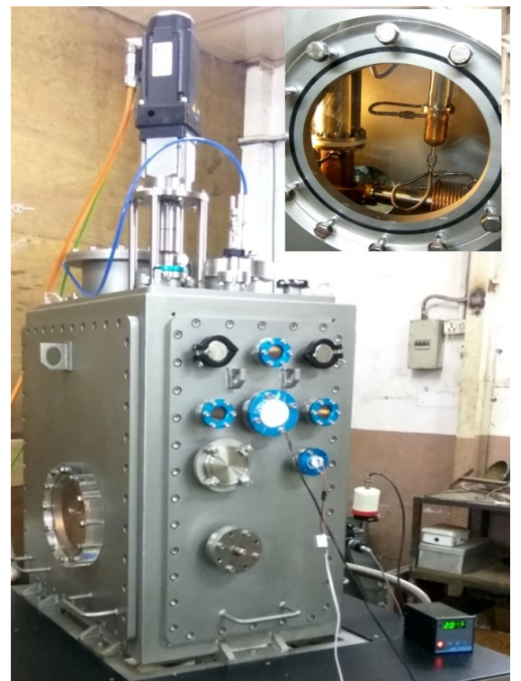
(L) Inside view of twin screw assembly and heat exchanger (R) The Cryogenic Twin-Screw Extruder System assembled with servomotor (Inset) View of the internal components through the view port.
