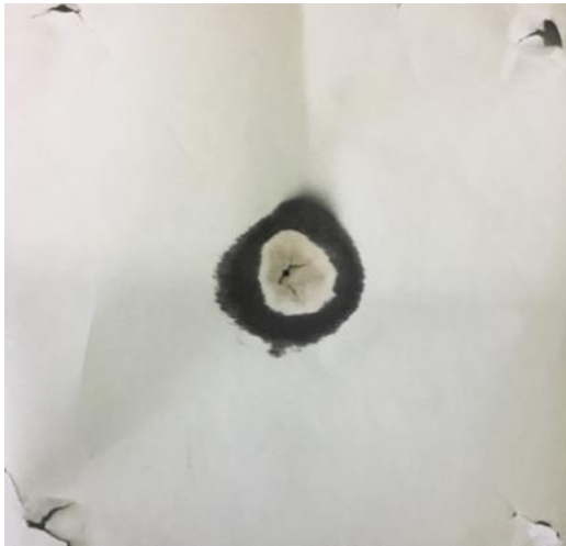
(L) Burn pattern at the exit of Gyrotron (R ) Waveforms of 500 kW-500 ms pulse from the Gyrotron
