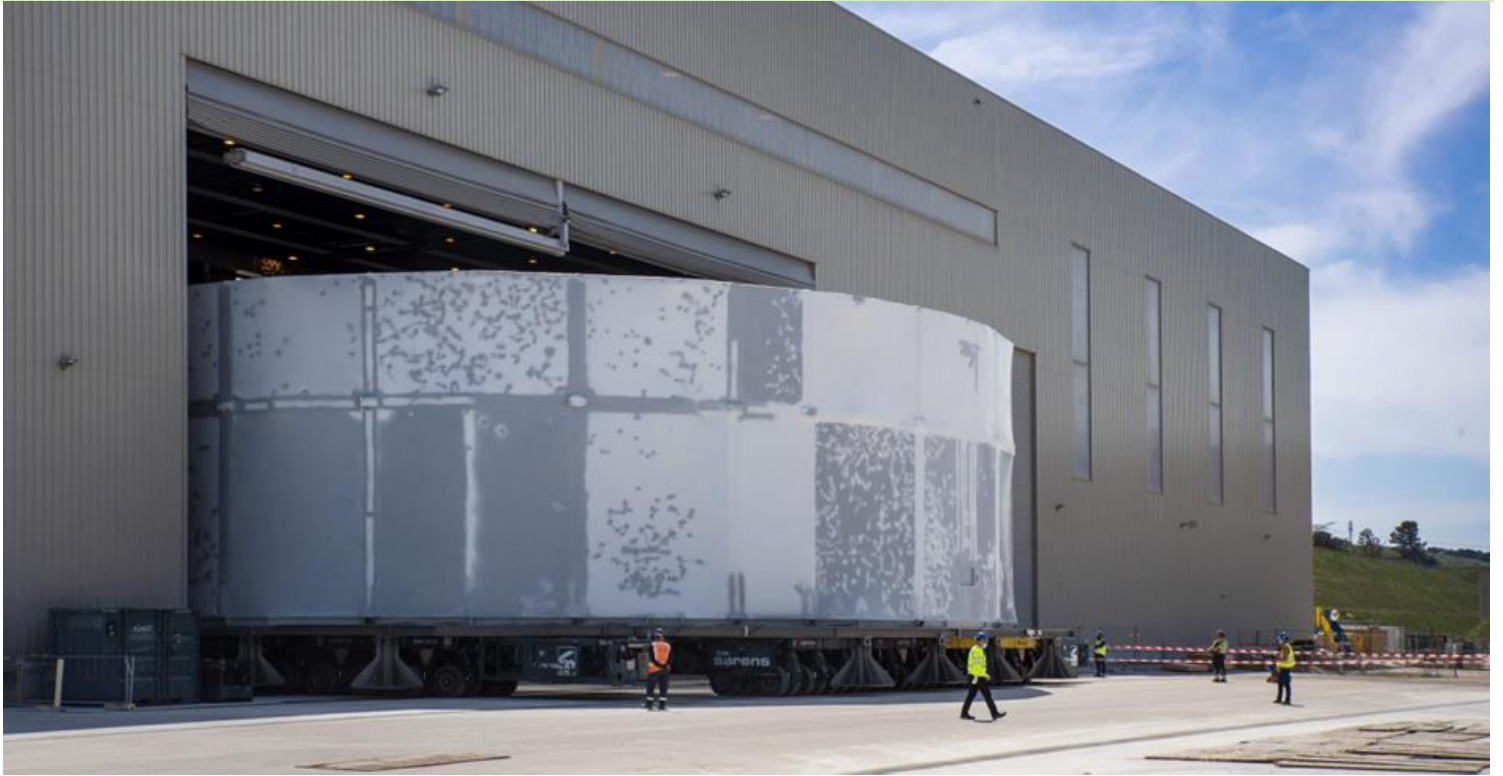
ITER Cryostat Lower Cylinder completed, wrapped and moved from Cryostat workshop to intermediate storage
