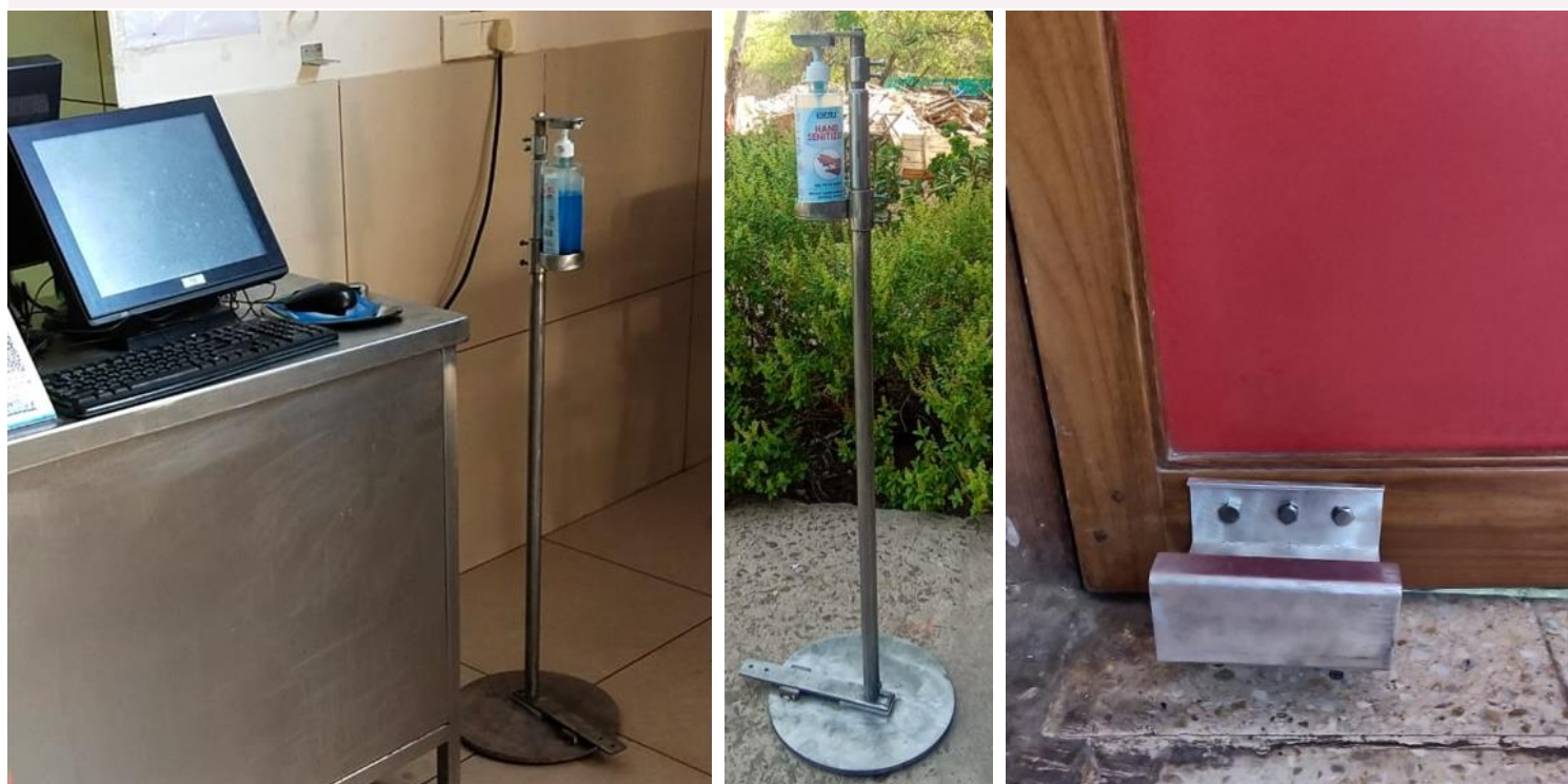
(L & M) The foot operated sanitizer dispenser (R) The foot operated door opener for doors, both designed and implemented by MESD and IPR Workshop.
