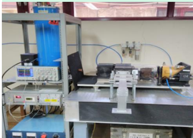
(L) The Michelson Interferometer System (M&R) Waveguide installation inside SST-1 hall (a) at radial port #12 (b) towards diagnostics lab
