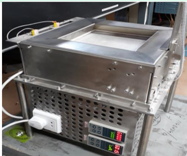
(L) The high temperature black body source with an operating temperature of 600°C (R) In-lab calibration of the Michelson Interferometer System.
