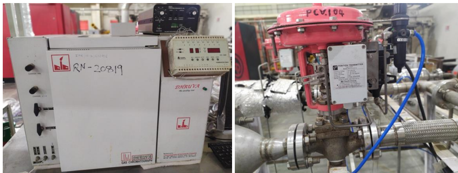
Indigenously developed (L) Oil content measuring instrument capable of PPB levels and (R) Pressure control valve for helium service with high leak tightness
