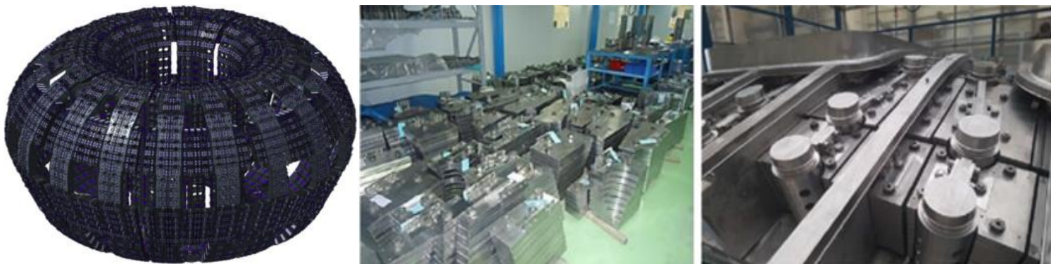
(L) 3D CAD model of the In-Wall Shield assembly; (M) The manufactured borated steel plate assemblies at M/s Avasarala, Bengaluru and (R) assembled in vessel sectors for ITER manufactured in Korea
