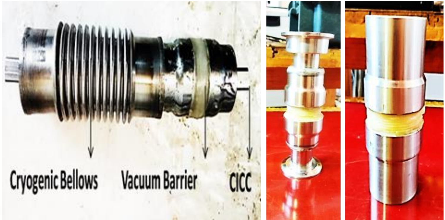
(Left) Vacuum barrier used in SC feeder (Right) Components of the indigenously developed vacuum barrier
