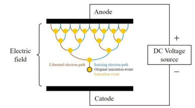
Application if electric field is the commonly used method in generating sustaining low temperature plasma. Any volume of gas has a few electrons and ions due to cosmic ray or radio active interactions within the gas. These get accelerated by the field and cause further ionization of neutral which in turn leads to avalanche of charged particles. A balance of loss and generation of charged particle ultimately lead to a steady-state plasma conditions.
