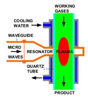
Microwave Energy transferred into electrons created by thermionic emission at typical frequency 2.45 GHz / 12.24 cm  $\lambda$  in different modes. High plasma densities of up  $10^{13}$ particle cm<sup>-3</sup> and temperatures  $\sim 10^3$  K achieved with higher electron temperatures
