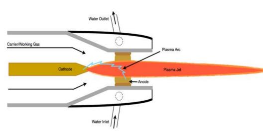
Thermal plasmas in Plasma Torches are achieved by DC,AC and RF currents and discharges in different configurations. Consists of electrodes of copper / tungsten graphite / molybdenum / silver etc. and plasma is formed from the continuously working gas /fluid. Thermal flowing efficiency of 90% is easily possible with power range from 1 kW tp 200kW at 6x10<sup>3</sup> to 50x10<sup>3</sup> K over a range and type of sources.
