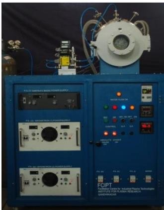
Magnetron Sputtering system in FCIPT
