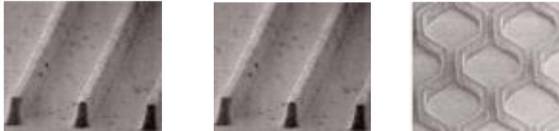
Examples of the barriers that isolate each cell. The distance between the walls of each cell is a couple hundred micrometers – or about ten times the diameter of a human hair
