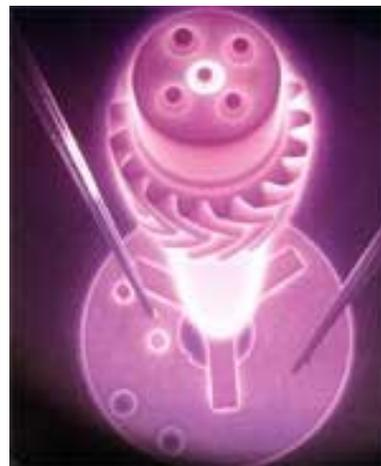
Figure1: (a) Experimental setup for Plasma Nitriding (b) Plasma Glow during Nitriding
