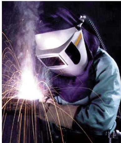
A welding helmet and flame retardant clothing protect a welder from sparks, heat and ultraviolet rays
