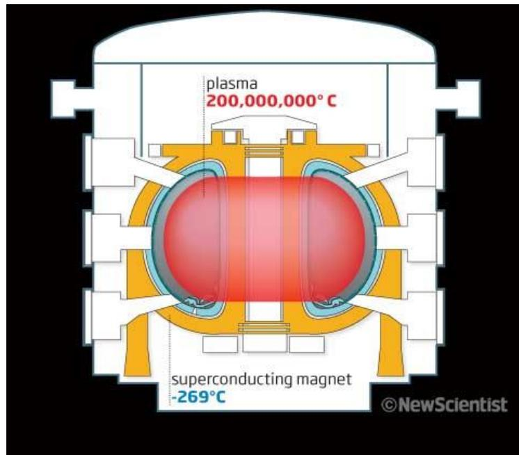
**Step 7.** Neutrons and other particles bombard the tiles on the plasma-facing components and heat them. In a future power station this heat will be harnessed to make electricity. Superconducting magnets operate near absolute zero. The distance to the magnets from the heart of the plasma sees the greatest temperature gradient in the universe.
