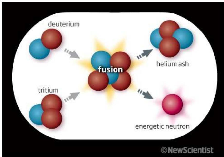
**Step 5.** To raise the temperature further, scientists fire radio and microwaves into the plasma and high-energy beams of deuterium atoms. The plasma then reaches 100 - 200 million °C, hot enough for the deuterium and tritium nuclei to fuse.
