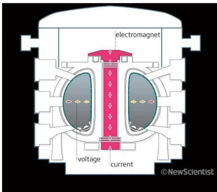
**Step 2.** Electricity flowing through this electromagnet (central solenoid) produces a voltage across the gas.
