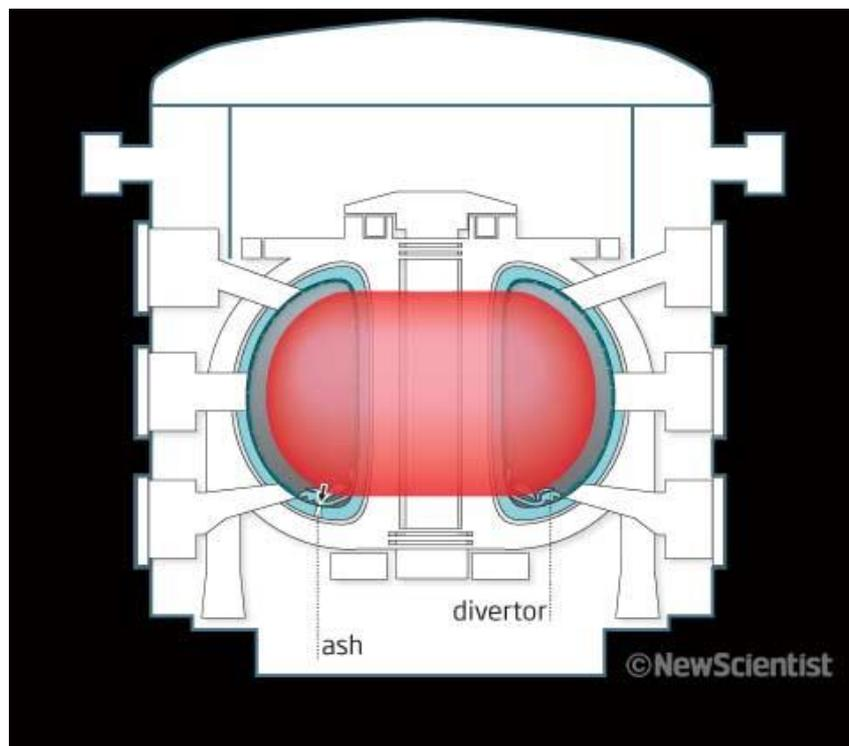
**Step 6.** Fusion produces high-energy neutrons and helium particles that deposit their energy into the plasma and keep it hot, before becoming “ash”. The “ash” is eventually forced out through the divertor.
