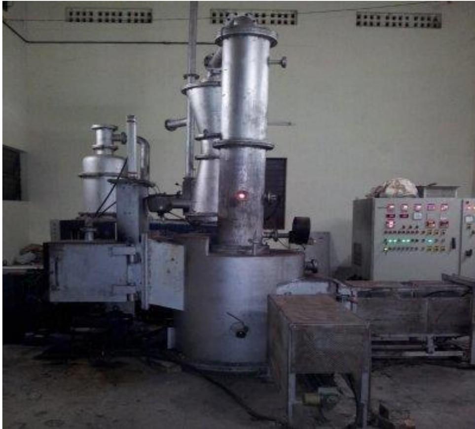
Plasma Pyrolysis Unit developed by FCIPT, IPR, Gandhinagar
