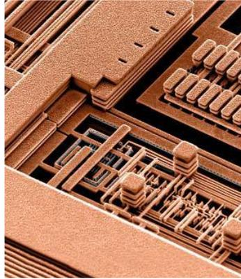
In this microscope photo of the wiring on a chip the smallest wires are more than 100 times thinner than a single hair
