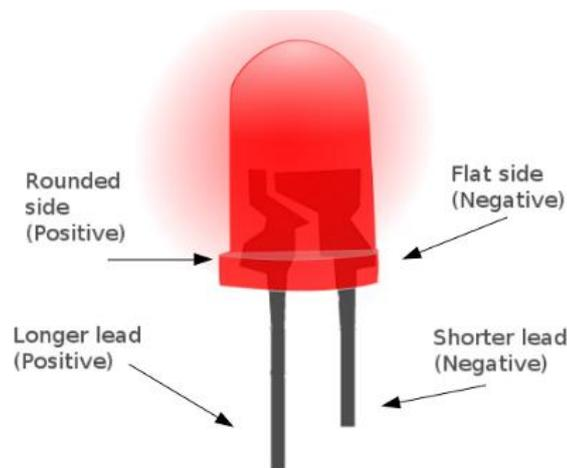
If the LED has two leads - one longer than the other - the longer lead is the positive (also known as the anode) lead. If the LED has two leads with leads that are equal in length, you can look at the metal plate inside the LED. The smaller plate indicates the positive (anode) lead; the larger plate belongs to the negative (cathode) lead. If the LED has a flat area (on the plastic housing), the lead adjacent to the flat area is the negative (cathode) lead.
