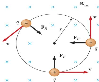
Consider a case of a positive charge moving in a uniform magnetic field. In the diagram, the direction of the magnetic field is into the paper ('x' denotes the backend of the arrow moving into the paper!). If a positive charge is fired, perpendicular to it, it will describe a uniform circular motion with the magnetic force described towards the centre of the circle. An electron would describe circular motion in the *opposite* direction.
