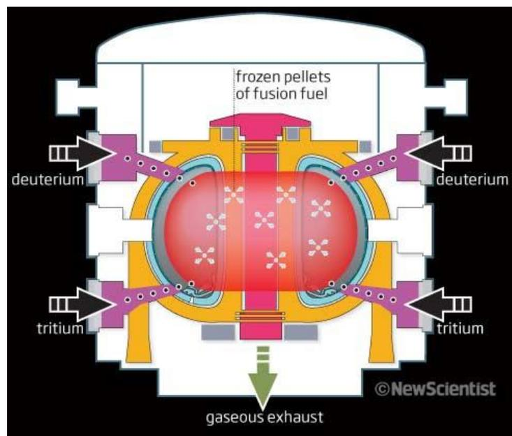
**Step 8.** The plasma must be continuously refuelled with deuterium and tritium for the process to continue. Unburnt fuel is also recovered from the gaseous exhaust and the reaction is fine-tuned by firing frozen pellets of fusion fuel deep into the plasma.
