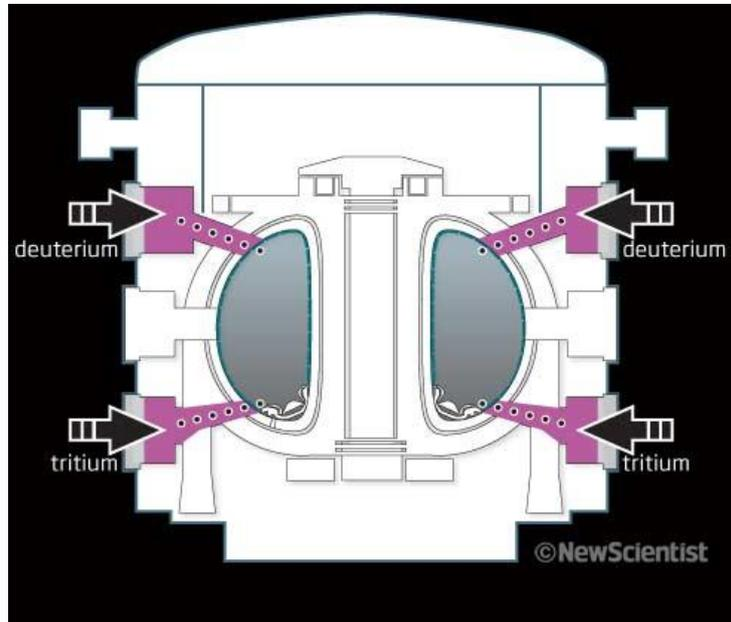
**Step 1.** Puffs of deuterium and tritium gas are injected into the donut-shaped vacuum vessel, called a Tokamak. The gas weighs less than a postage stamp and fills a volume one-third that of an Olympic swimming pool.
