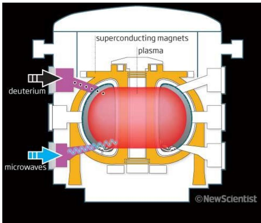
**Step 4.** Plasma is locked inside the vacuum vessel by magnetic fields that are created by an array of superconducting magnetic coils. The magnetic coils generate a current in the plasma
