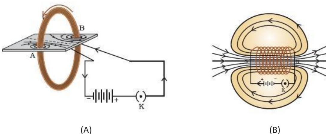
(A) Magnetic field produced by a current carrying circular coil, and (B) Field lines of the magnetic field through and around a current carrying solenoid
