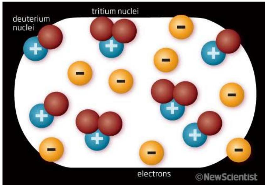
**Step 3.** Voltage rips electrons from the deuterium and tritium atoms. They turn into charged atoms (ions) within a few microseconds, forming a particle soup called a plasma.
