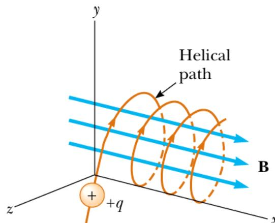
Take wire (or the soft spring) given in the kit and make it into a spiral. Ask your friend to pass a rod through the spiral and hold it firmly denoting the direction of magnetic field  $\mathbf{B}$  as shown in the figure. Now pass a bead through the wire and slide it along the wire as shown in the figure. The bead denotes a positive charge that moves along a helical path in the direction of
