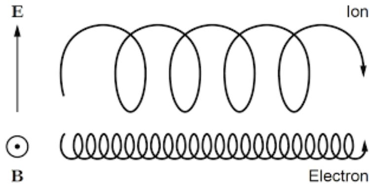
Using the given plastic (or metallic) wire, with  $E$  and  $B$  representing electric and magnetic fields along the Z and X directions, show the paths of ions and electrons as they drift in the YZ-plane along the Y direction.
