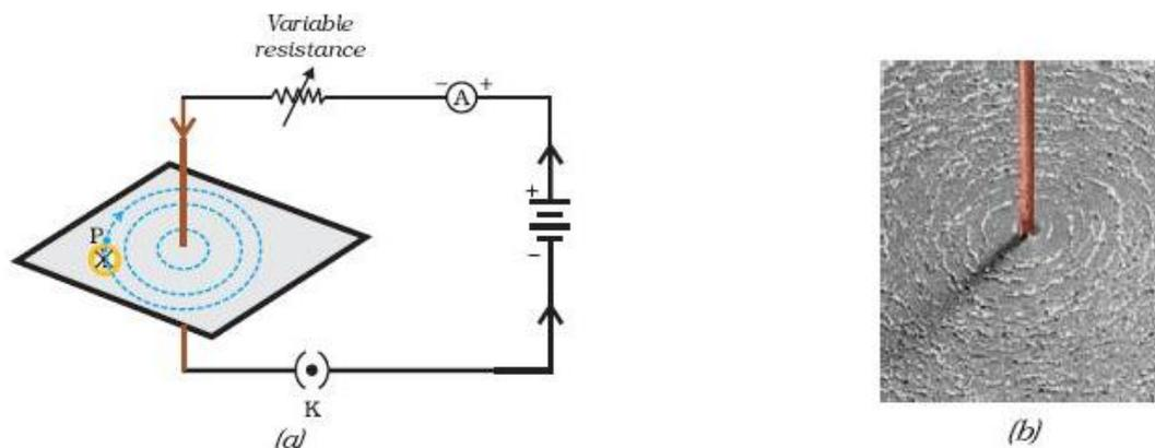
(a) A pattern of concentric circles indicating the field line of magnetic field around a straight conducting wire. The arrow in the circles show the direction of the field lines. (b) A close up of the pattern obtained.
