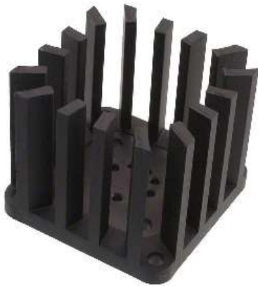
HEATSINK 8P TO-3 4.5C/W Heat Sink TO-3 Aluminium 10W @ 50°C Board Level
