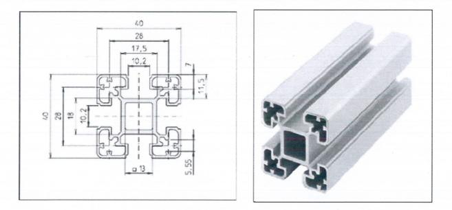
Sr. No: 1 Dimensions : Aluminium square section 40 mm X 40 mm X 3000 mm cross sectional view (All dimensions in mm typical) –typical cross sectional view (indicative)
