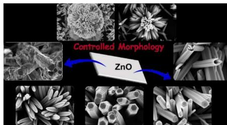
Fig. 1. Controlled morphology of ZnO nanostructures from flowers to rods to tubes
