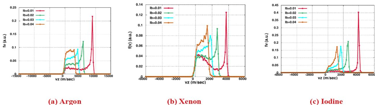
Figure 2: Ion velocity distribution function at  $z = 0.07\text{m}$  for argon, xenon and iodine, where fuel gas neutral pressure is fixed at 1.23 mTorr. A directed ion beam having velocity around 9km/s for argon plasma, around 4km/s for xenon and iodine plasma case are observed.
