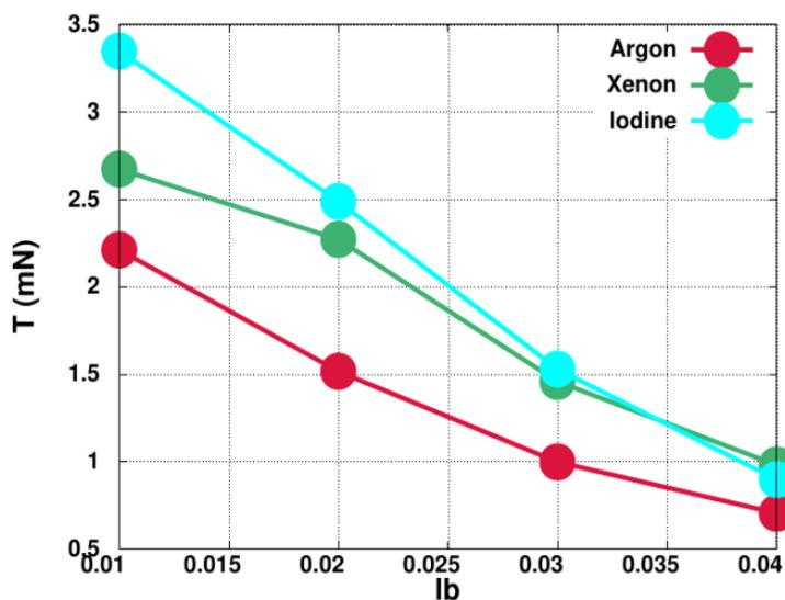
Figure 3: Net plasma thrust profile with different magnetic field divergence for argon, xenon and iodine fuels.
