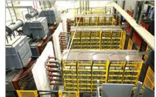
Power supply test bed, EC, IC and DNB power supplies
