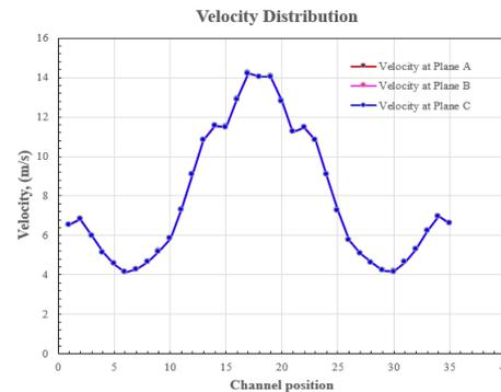
Fig. 5 Plot of average velocity distribution at the plane A, B, and C.
