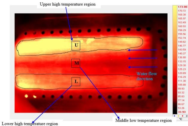
Fig.6 IR image of temperature distribution over the surface of the OFE copper
