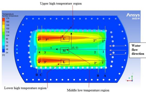
Fig. 4 Results of surface temperature distribution over OFE copper plate surface using 3D CFD BP model.
