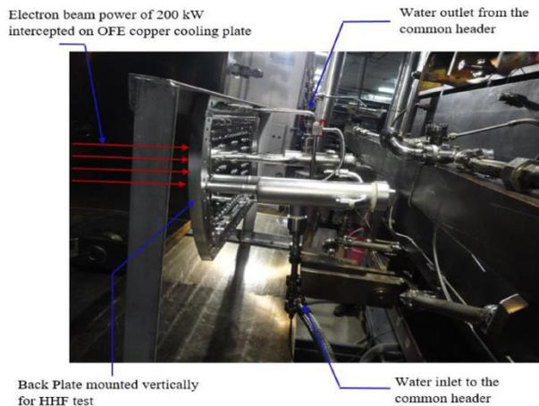
Fig.2 Back Plate assembled in Vacuum chamber at HHFTF Center, IPR.
