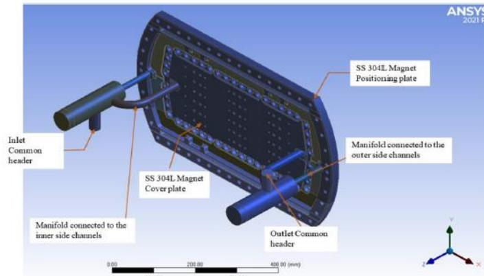
Fig.3 3D CFD model of the actual sized back plate
