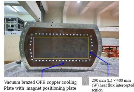
Fig. 1 (a) Fabricated Back Plate (b) Vacuum brazed OFE copper cooling plate with heat flux intercepted area.
