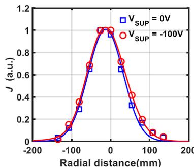
Radial profiles of ion current ( $V_{SUP} = -100 V$ ) and electron current ( $V_{SUP} = 0 V$ ) in the beam
