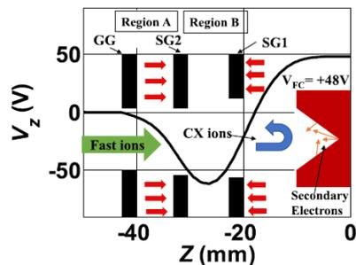
Schematic of Faraday cup with filletting electrodes
