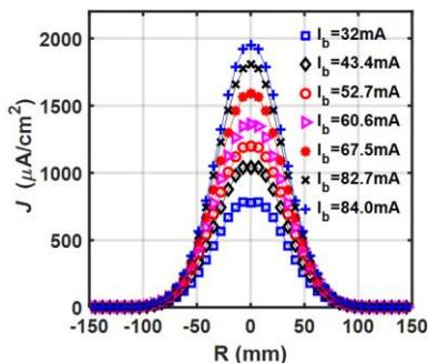
Radial profiles of ion current density for different Beam currents
