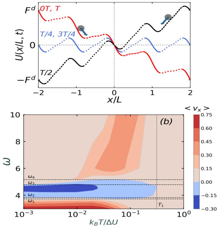
Figure Caption: (top) Pictorial representation of the rocking ratchet,  $U(x, t) = U(x) - A_d \cos(\omega t)x$  (bottom) Contour plots of average velocity as a function of translation noise  $k_B T / \Delta U$  and driving frequency  $\omega$ .
