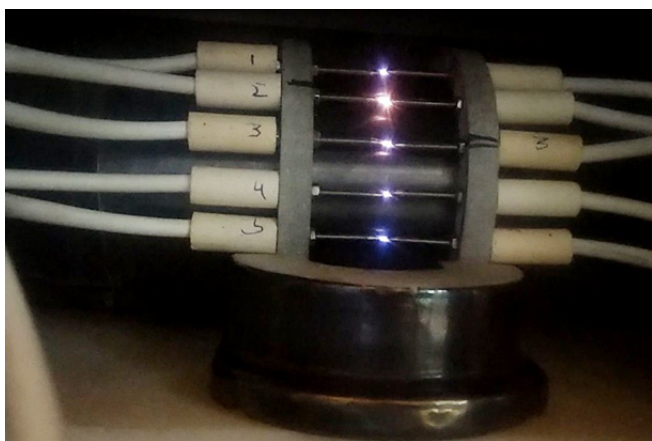
Figure A.3.2 CO 2 Plasma Generated for Nodular Corrosion Studies
