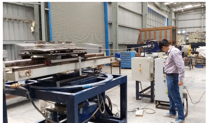
Figure A.2.2. Special Purpose Winding Machine for saddle shape coil
