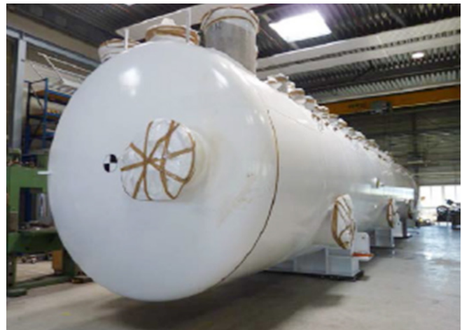
Figure B.4 Cryoplant Termination Cold Box (CTCB) Vacuum Shell
