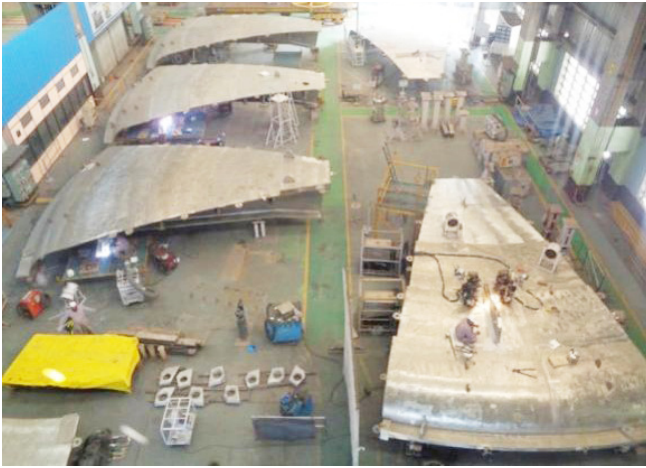
Figure B.2 Manufacturing of Top Lid segments nearing completion at Hazira, India
