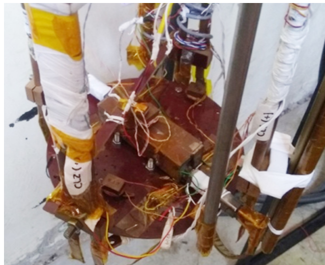
Figure A.4.1.2 Hybrid Joint integrated with the test insert
