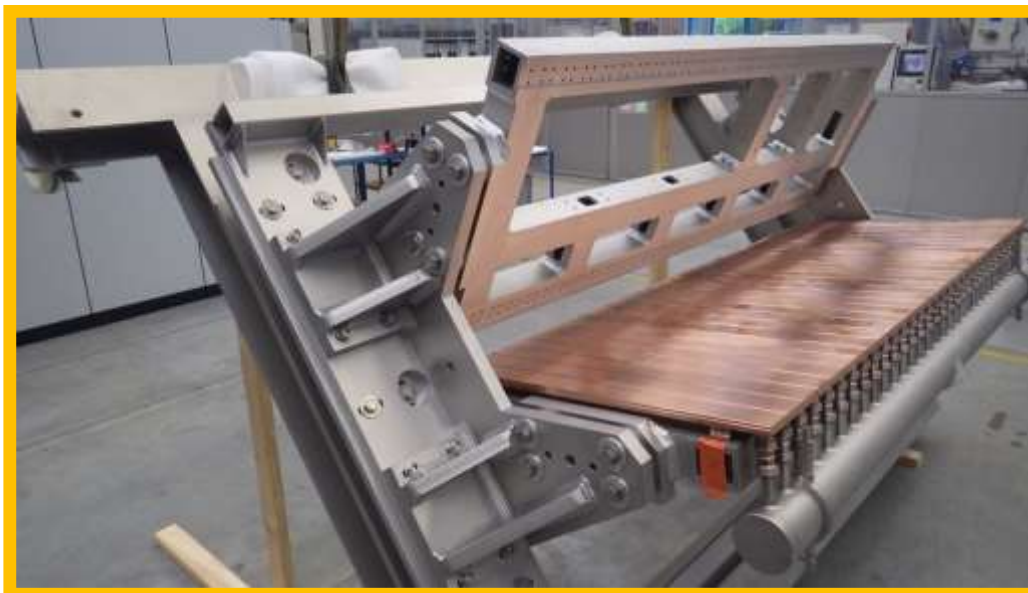
Figure 6 Assembly of left arm heat transfer elements for SPIDER beam dump for Diagnostic Neutral Beam for ITER
