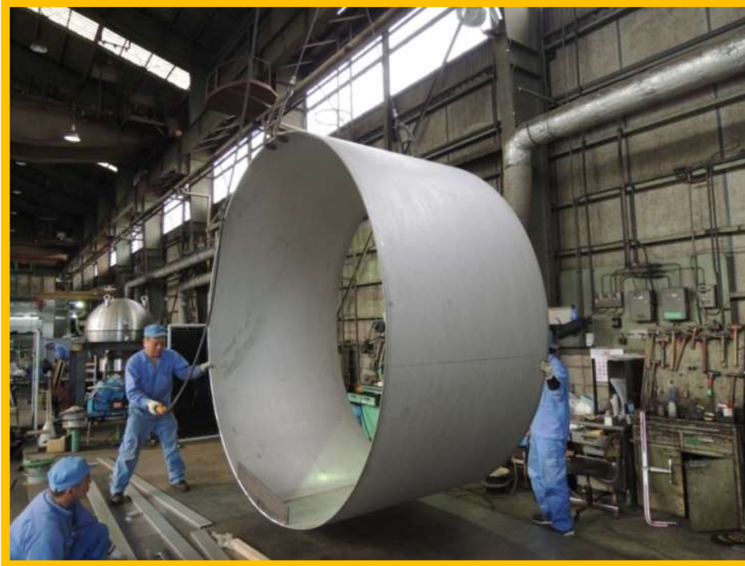
Figure 5 Manufacturing process of shell for cryo-distribution and cryo-lines
