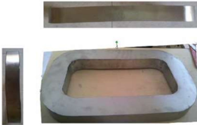
Figure 2. A 1:1 prototype of the ELM coil case after successful technology validation
