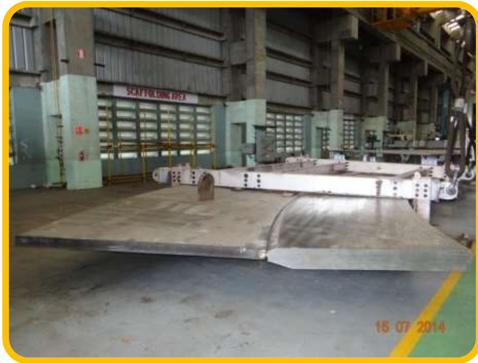
Figure 4 Cryostat Manufacturing process – bottom plate and horizontal plate
