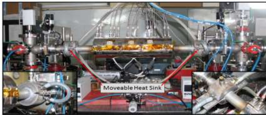
Fig: A new HPO with movable heat sinks on either side. The inset shows the moveable heat sink in the system.
