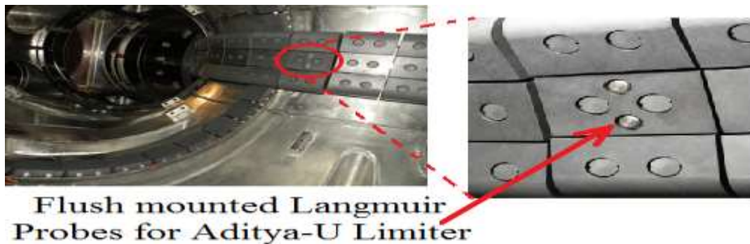
Fig: Flush mounted Langmuir probes installed on the belt limiter on the inboard side of the Aditya-U tokamak.
