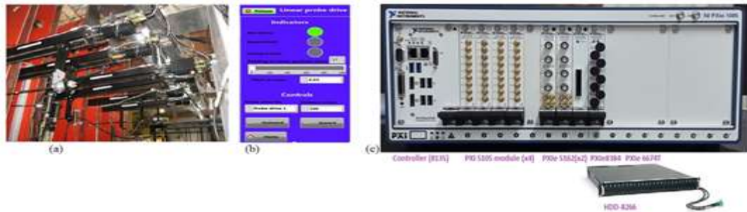
Fig: a) probe positioning system, 2) data logger for PPS and 3) 40 channel data acquisition system commissioned in LVPD.
