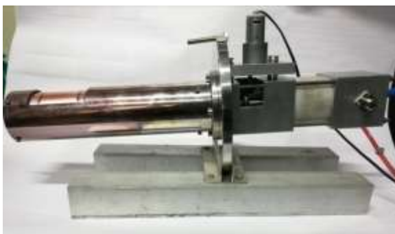
Figure 3a:-Rotatable Magnetron Developed at IPR
