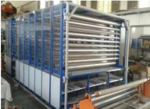
Figure 2a: Plasma system for In-line textile treatment
