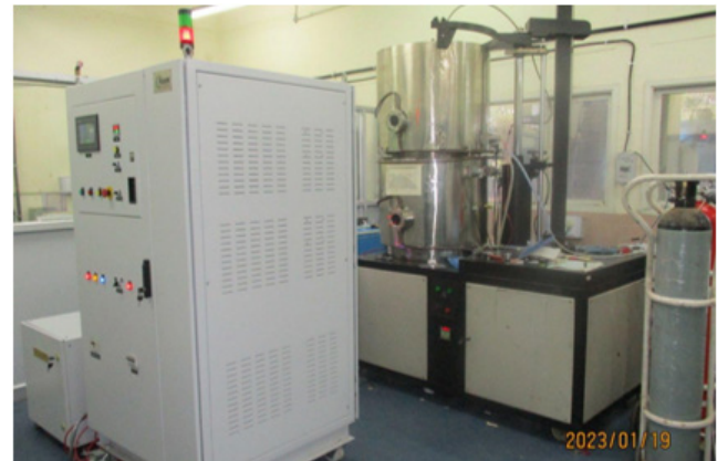
Figure A.4.24: Pulsed HV DC power supply integrated with plasma nitriding system at IGCAR, Kalpakkam.
