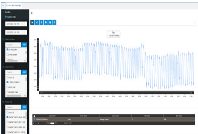
Figure D.5: Datacentre 24 hour Average Current (EMS).
