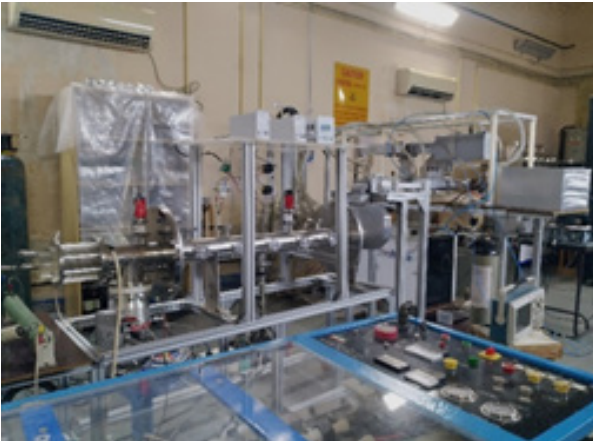
Figure A.2.23: HPM – plasma coupling set-up with the 3 MW, 3 GHz pulsed magnetron source coupled to a 100 mm plasma column.
