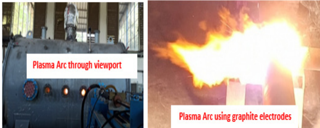
Figure A.1.5: 100kW plasma arc system.
