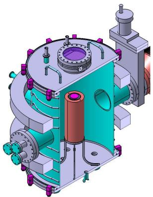
Figure 3: Arrangement of Heater, Substrate Pipe and Cathode in Vacuum Chamber
