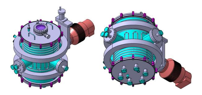
Figure 1: Conceptual 3-D Model of Sputtering system
