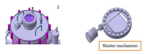
Figure – 4: View port along with the shutter mechanism
