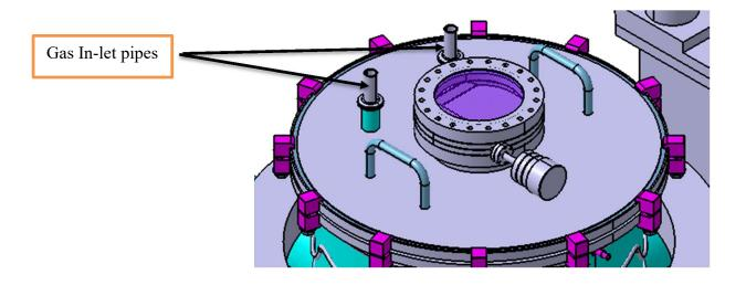
Figure – 5: Arrangement of gas in-let pipes on top flange
