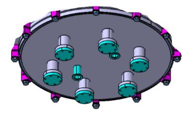
Figure – 6: Bottom flange along with CF flange and KF Couplers
