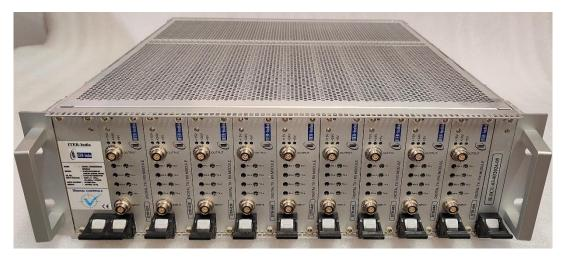
OptoSIGN™ Signal Conditioning Modules (SCM) are used for interfacing different sub systems to data acquisition & control system providing optical isolation. It also reduces EMI Interferences i.e. provides minimal emission & better immunity from conductive or radiative coupling. OptoSIGN™ has generic specification to match various applications. There are three types of OptoSIGN™ modules are developed.
