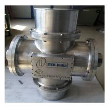
The RF coaxial switches are multi-port devices mainly used in VHF (Very High frequency) and UHF (Ultra High Frequency) range for switching the transmission of RF power towards various loads. A motorized section of switch is used to connect and disconnect various loads to transmit RF power.
