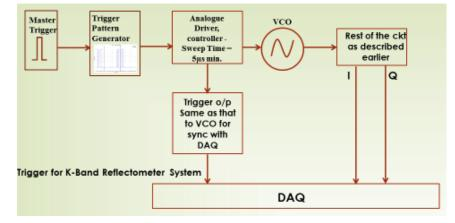
The trigger pattern generator should accept a custom txt/csv file containing arbitrary trigger pattern with programmable time axis. Sample trigger patterns are shown below.
