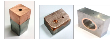
Reference standard for various metallic joints
