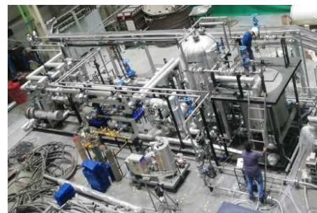
High Pressure High Temperature Water Circulation System (60 bar, 160C, 300 lpm)
