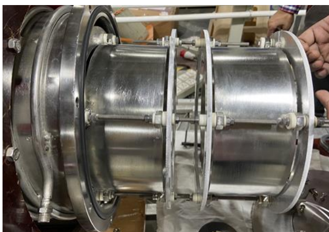
(L) Electrode assembly of Capacitive-Coupled RF discharge (M) Inside view of BEAM setup showing the cylindrical discharge electrodes (R) Ring-shape hot plasma produced by cylindrical RF discharge with axial magnetic field.
