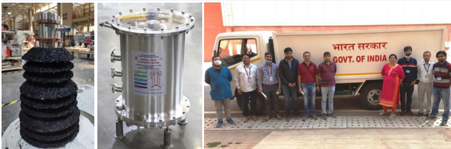
(L) Inner assembly components of CVPS (M) Cryogenic Vacuum Pumping System -Model no. IPR-CP400-Air-80 (R) The cryopumps being dispatched to SAC-ISRO
