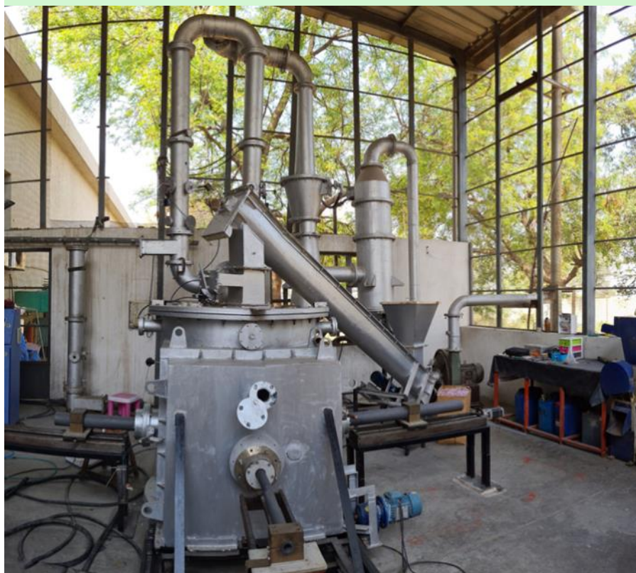
The R&D prototype of the high capacity plasma pyrolysis system at FCIPT
