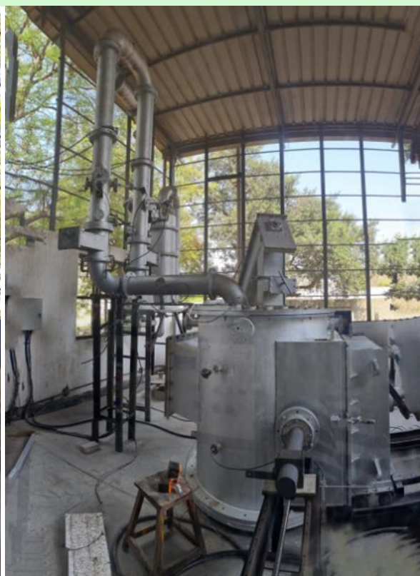
The R&D prototype of the high capacity plasma pyrolysis system at FCIPT
