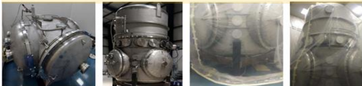
HAM & BSC chamber Assembly ready for He leak test, UHV compatible plastic hoods used for gross leak testing and subsequently for vacuum demonstration
