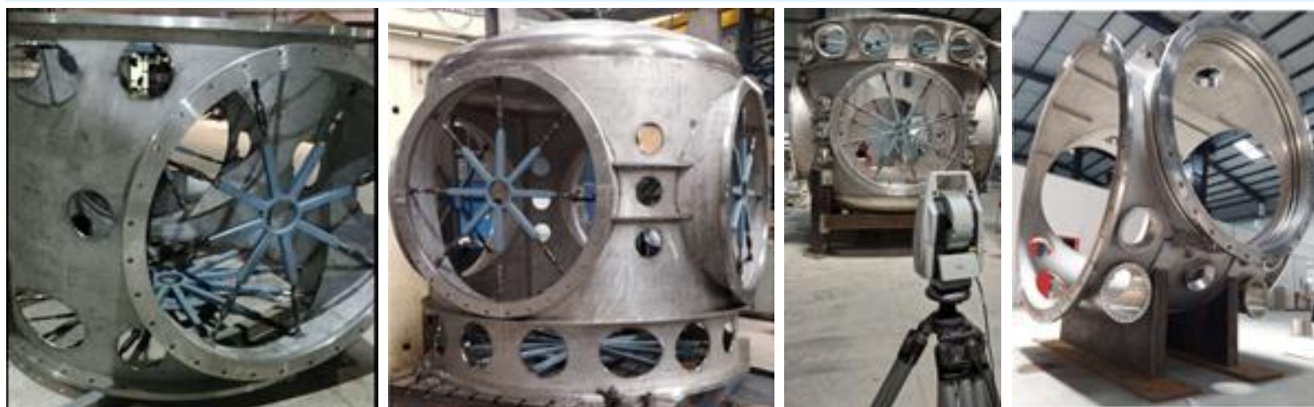
BSC and HAM chambers fabricated at VTPL, Bengaluru. Metrology performed using laser tracker, subsequently steam-cleaned.
