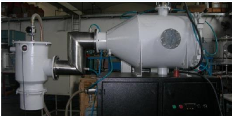
(L) Plasma-based nano-materials synthesis system at FCIPT campus (R) The plasma produced inside the system.
