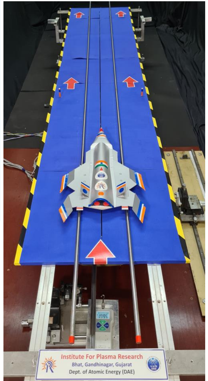
(L) The prototype system showing the LIM and the load (R) The model aircraft being launched using the system
