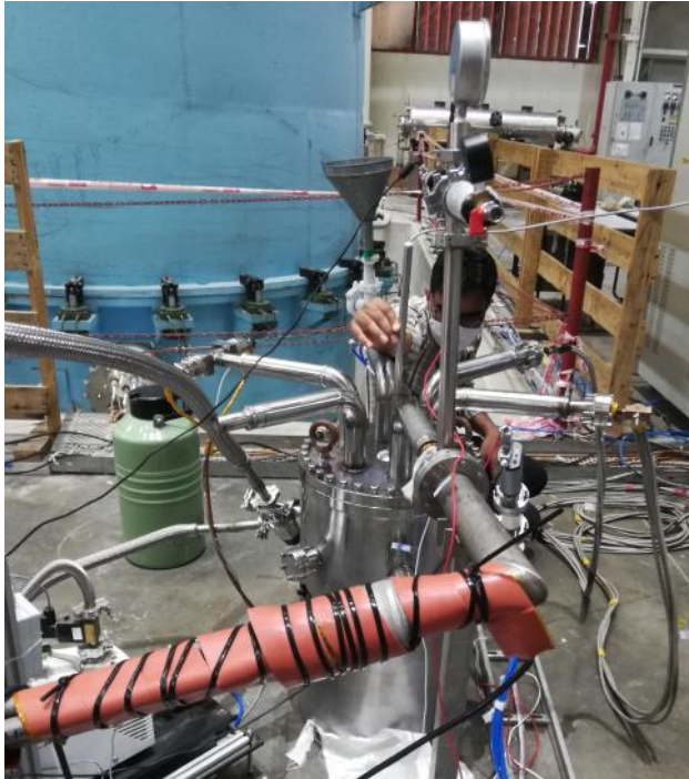
(L) The HTS coil during testing with its housing cryostat (R) Measured Magnetic field at operating currents
