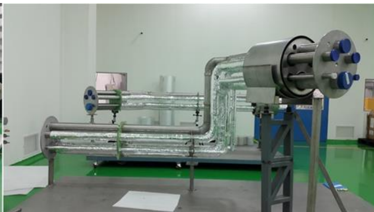
Multi-process pipe cryoline under manufacturing and assembly at M/S INOXCVA , Vadodara
