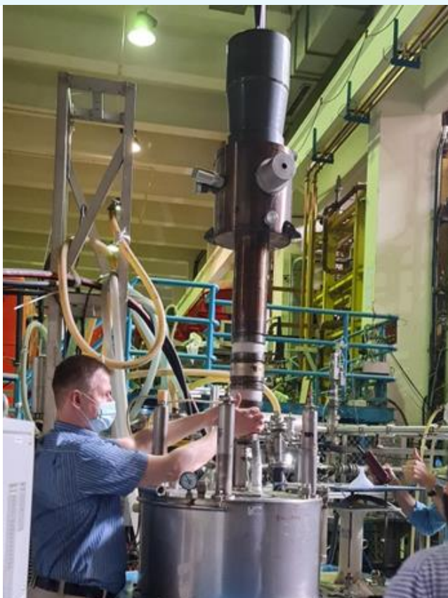
(L) The Gyrotron being installed (R) Connecting the Gyrotron to the transmission line
