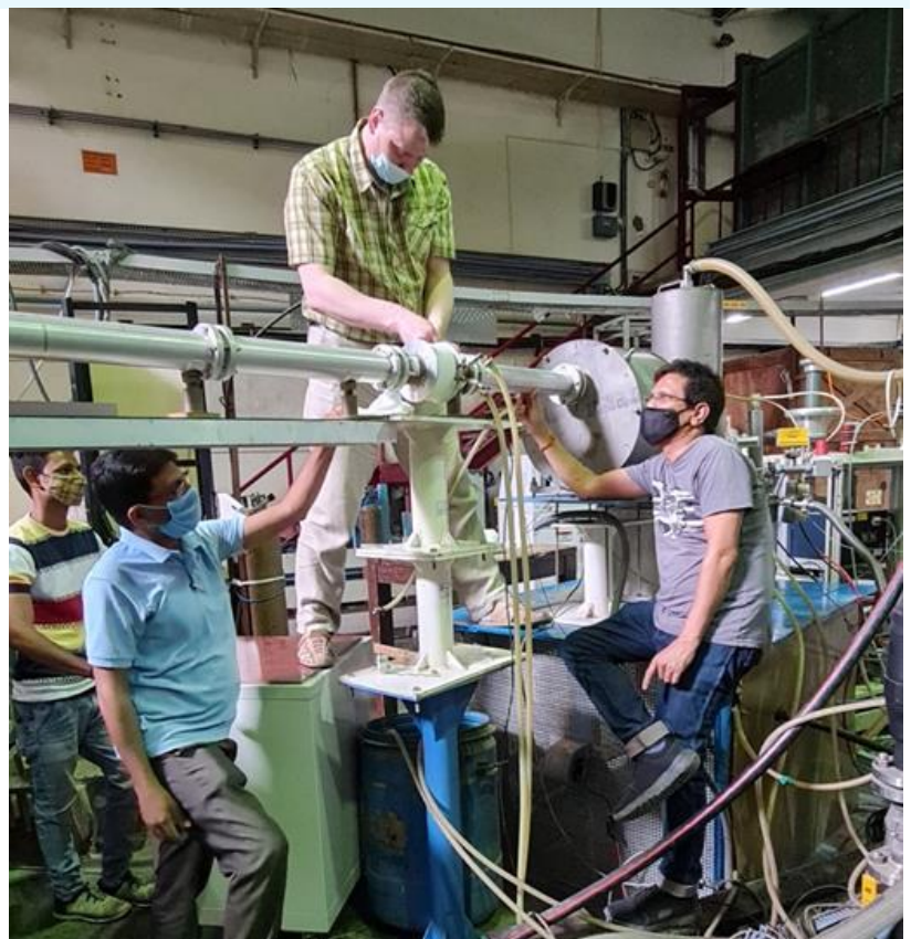
(L) The Gyrotron being installed (R) Connecting the Gyrotron to the transmission line
