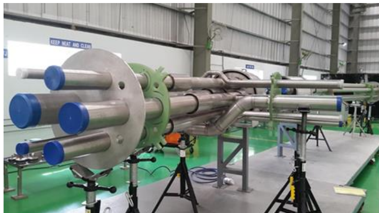
Multi-process pipe cryoline under manufacturing and assembly at M/S INOXCVA , Vadodara
