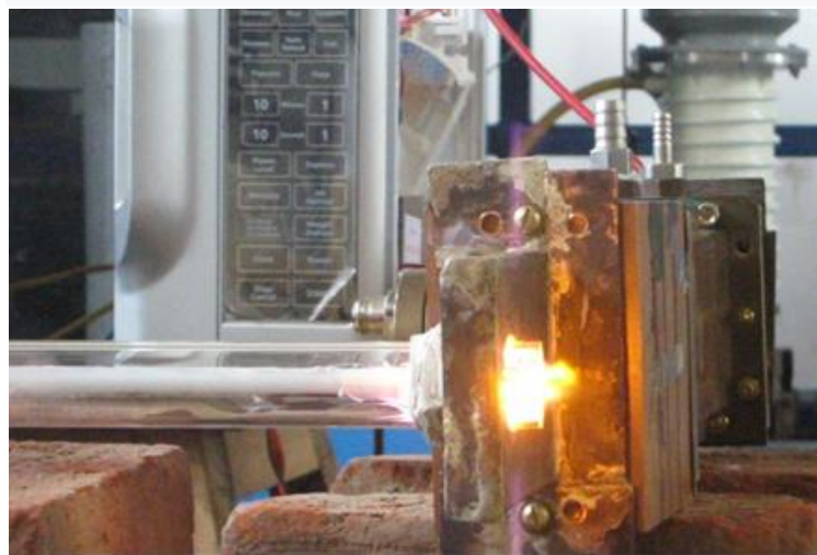
(L) Microwave plasma arc at atmospheric pressure (R) Microwave plasma coupled to a low pressure fluorescent tube
