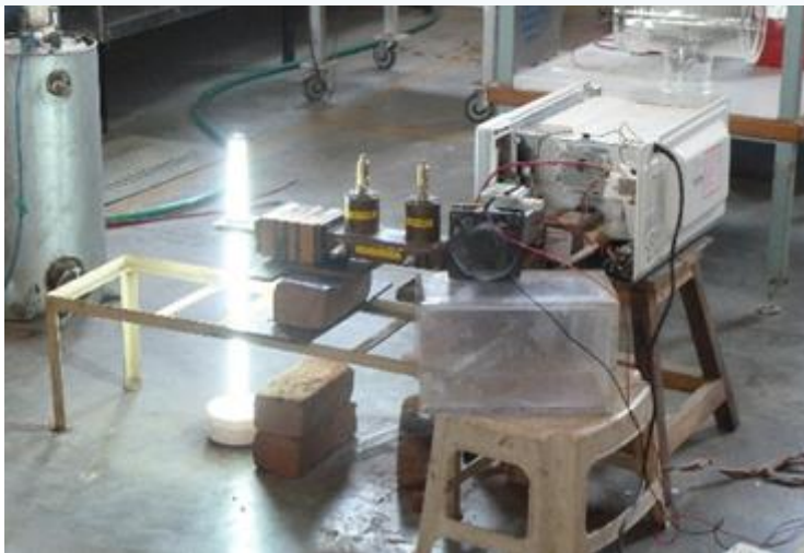
(L) Microwave plasma arc at atmospheric pressure (R) Microwave plasma coupled to a low pressure fluorescent tube
