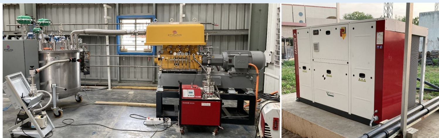
(L) The SPC-4 Cryogenerator with cryostat and five cryofans (R) Chiller for the Stirling Cryocooler (SPC-4)
