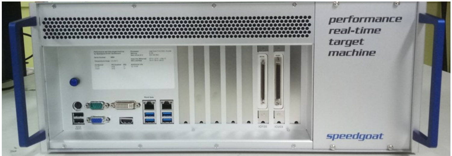
(Top) Schematic (bottom) Hardware for the of the HIL testing system to be implemented on SST-1
