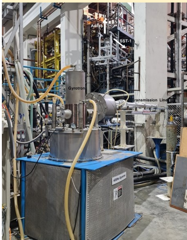
(L) The 42GHz-500kW ECRH system (R) The ECRH system on Aditya-U
