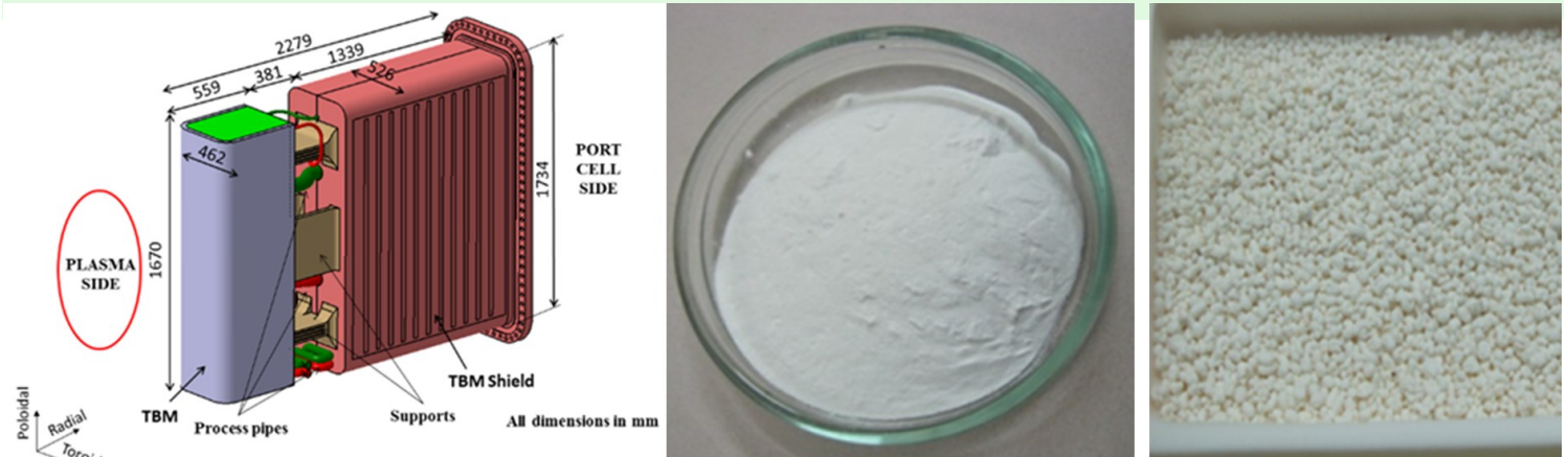
(L) The LLCB TBM set (R) \text{Li}_2\text{TiO}_3 powder and pebble prepared at IPR
