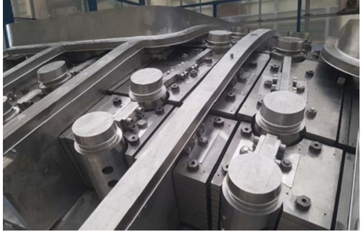
(L) In-wall shield blocks supplied by India under installation in the vacuum vessel sectors in Korea
