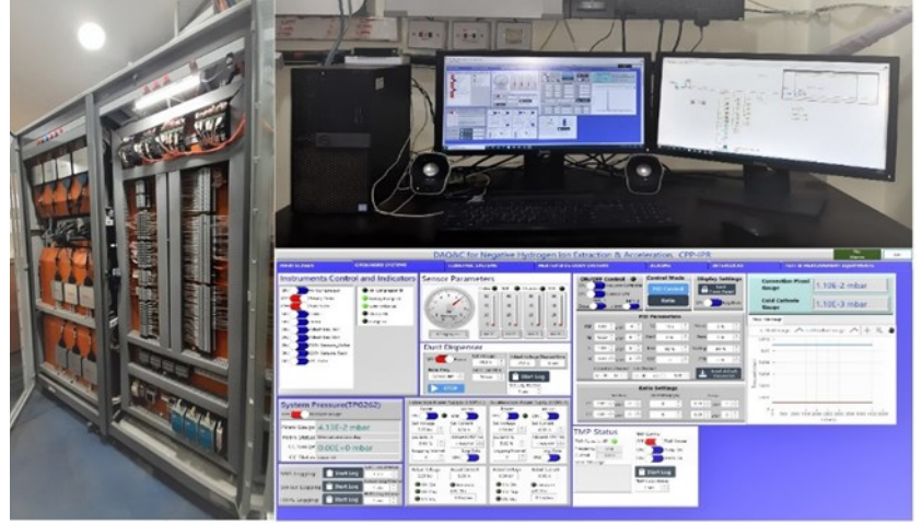
(L) The negative hydrogen ion extraction system and HV power supplies (R) PXI based DAQ & control system
