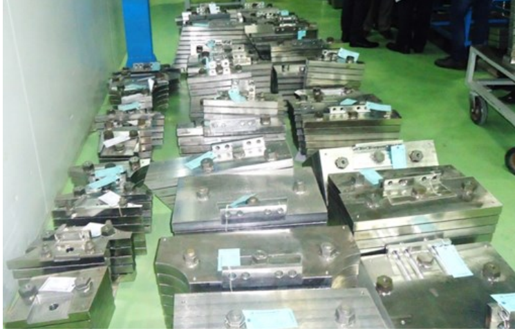
(L) In-wall shield blocks supplied by India under installation in the vacuum vessel sectors in Korea
