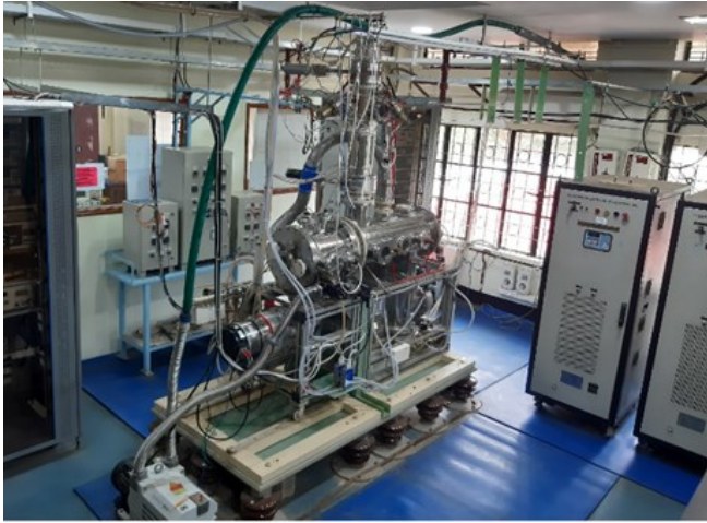
(L) The negative hydrogen ion extraction system and HV power supplies (R) PXI based DAQ & control system
