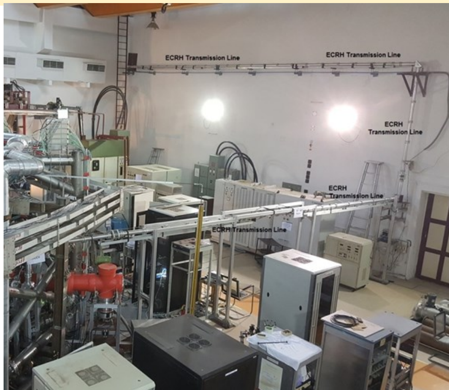
(L) The 42GHz-500kW ECRH system (R) The ECRH system on Aditya-U
