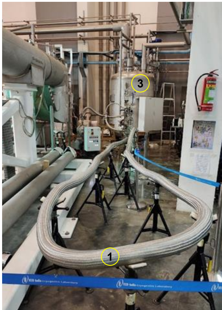
External view of the interface coupler (1) Mockup of the DMS cryoline (2) External interface coupler (3) 80K cold box (4) Internal of interface coupler
