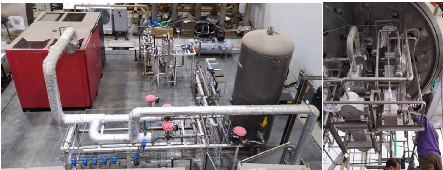
(L) Indigenously developed helium compressor and oil removal system (R) Components of the cold box being assembled.
