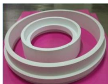
Clockwise : BN/Silica composite liners, the 300mN SPT and handing over ceremony in the presence of Director, VSSC
