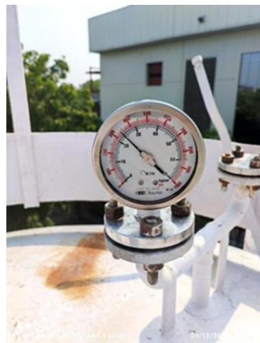
(L-R) : High pressure and medium pressure storage vessels; Hydro test pressure @ 203.5 bar (g) and at 23.4 bar (g)
