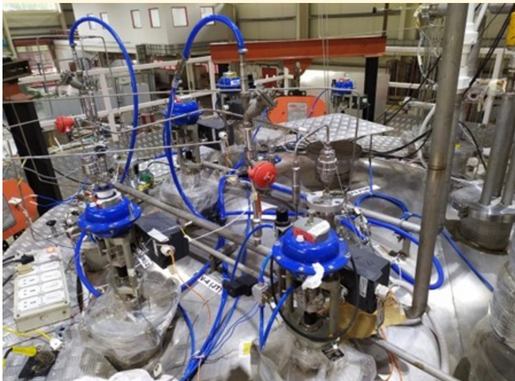
(L) the high speed turbines integrated with the cold box (R) The indigenously developed helium circulator
