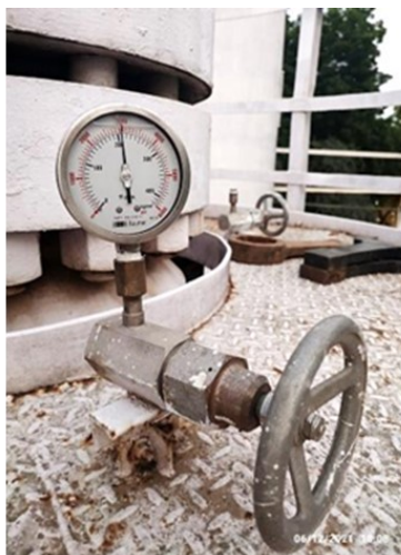
(L-R) : High pressure and medium pressure storage vessels; Hydro test pressure @ 203.5 bar (g) and at 23.4 bar (g)
