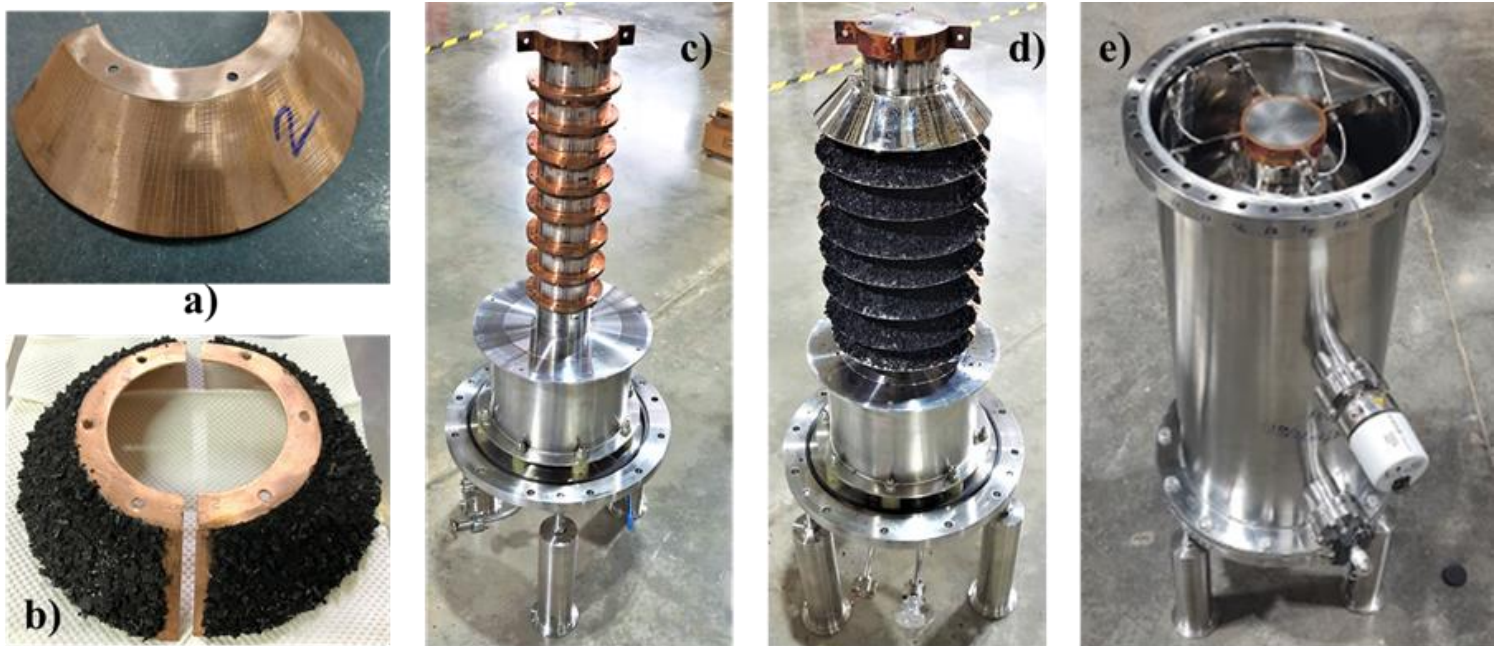
(a) Bare copper panel half (b) Pair of charcoal coated panel (c) SS bath and copper collar rings, (d) charcoal coated panels assembly and assembled cryopump (kept inverted)
