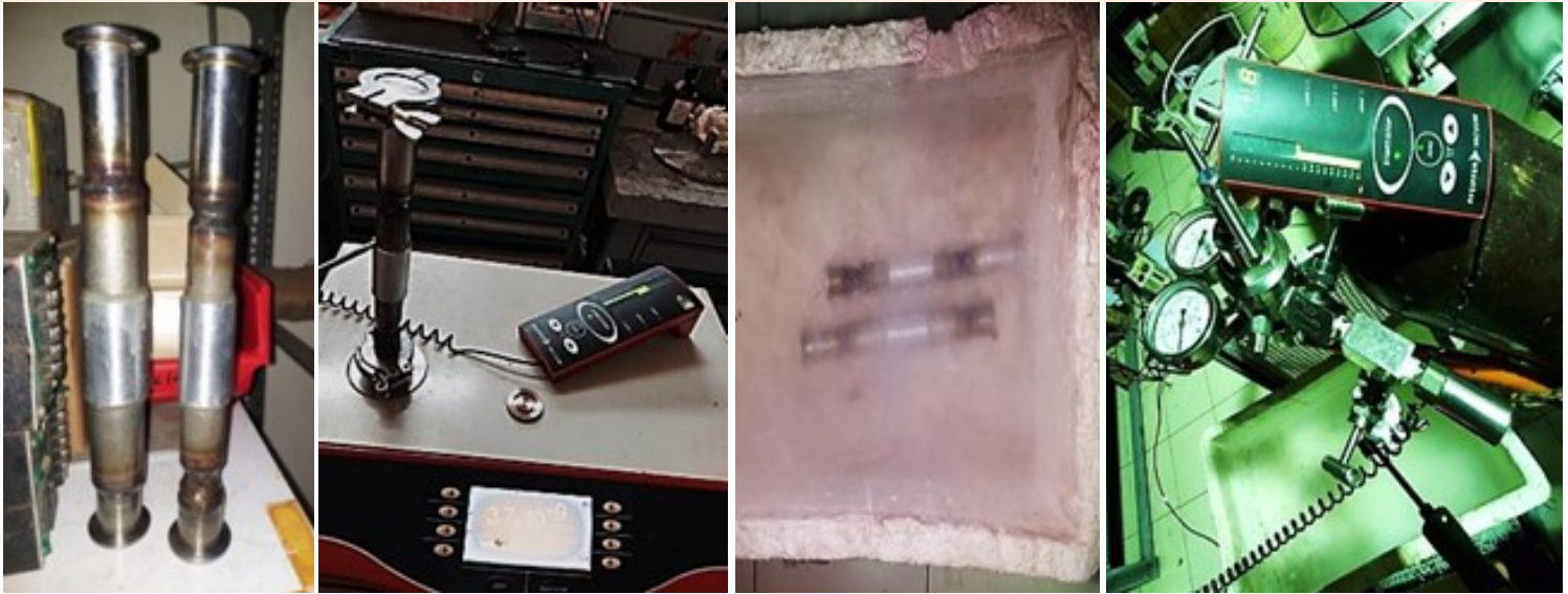
(L-R) Developed Bi-Metallic Joints ; He leak test at 300 K 3.7 \times 10^{-09} mbar l/s ; Thermal shock test (dipped) at 77 K; Helium leak test (sniffer) @ 10 bar (g), 77 K
