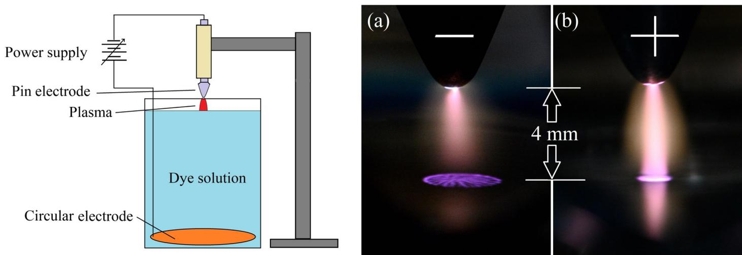
(L) Schematic diagram of APGD plasma set up (R) Photographs of APGD plasma operated in (a) liquid anode and (b) liquid cathode mode.
