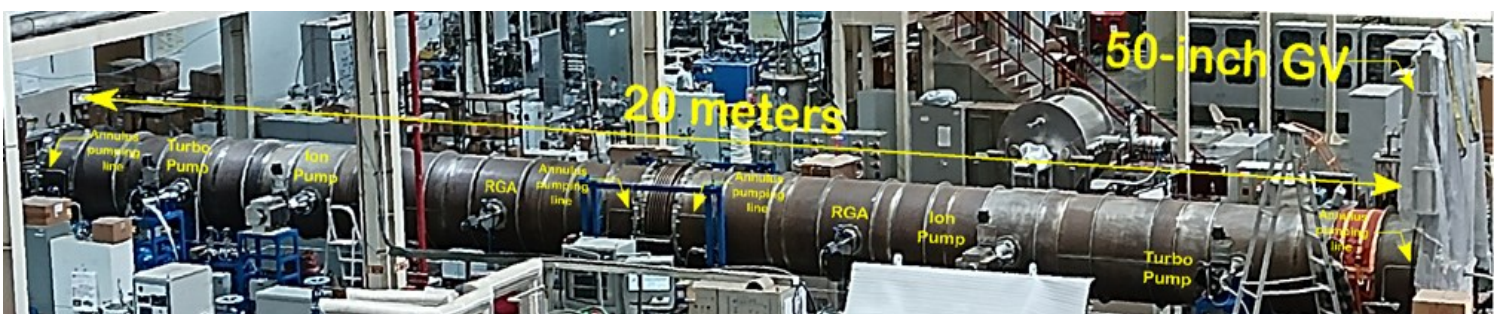
The LI-VISTA vacuum vessels being assembled in the IPR New Laboratory Building
