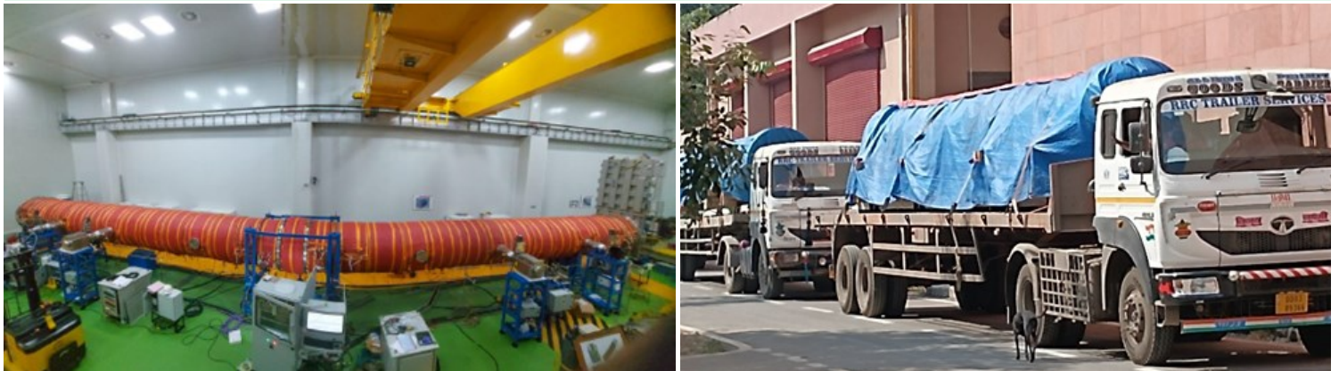
(L) Testing of the Integrated Vacuum Vessel at the factory (R) The vacuum vessels transported to IPR by road from Mumbai
