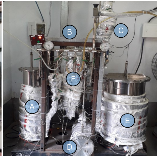
(L) MHD experimental loop at IPR (R) Indigenously developed Pb-Li production system (A) Li tank (B) Mixing vessel (C) Pb measuring vessel (D) Drain tank (E) Pb tank (F) Li nozzle
