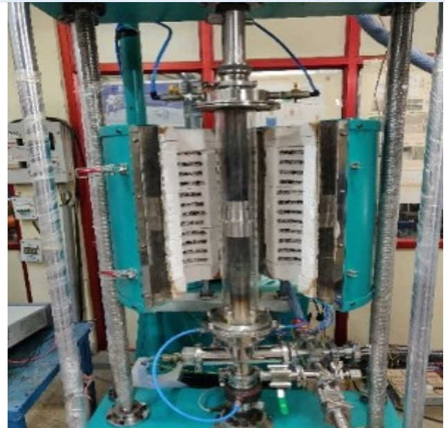
(L) EHCL system at IPR (R) Thermo-mechanical test facility for pebble beds measurement
