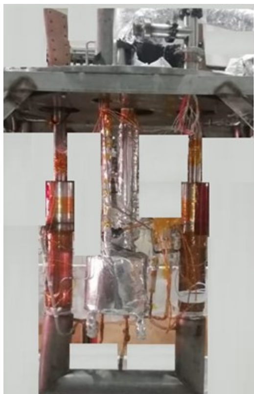
(L) HTS CL equipped with all instruments on test stand (R) Temperature evolution during current charging at different superconducting joints section.
