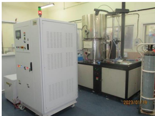
(L) The specifications of the Pulsed HV DC power supply (R) High voltage power supply integrated with Plasma Nitriding System at IGCAR Kalpakkam
