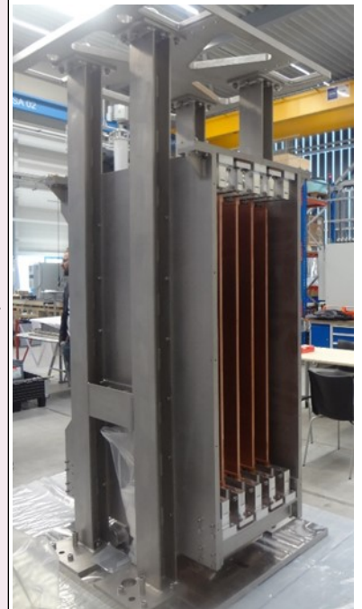
1 m long, 1.8 m high, 5 ton, Residual Ion Dump consisting of an assembly of 50 individual water cooled elements of CuCrZr to separate ionic component of the beam from the neutrals. Alternate panels of the assembly at high voltage and ground potentials.
