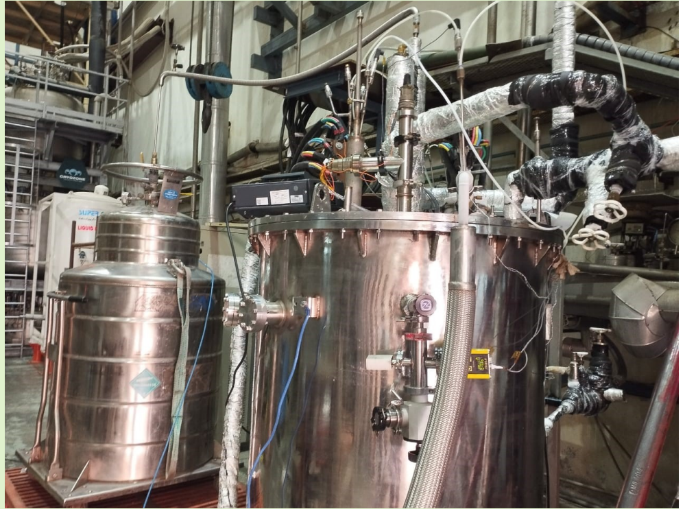
HTS CL test cryostat equipped with necessary instrumentations along with liquid helium Dewar connected to the test assembly
