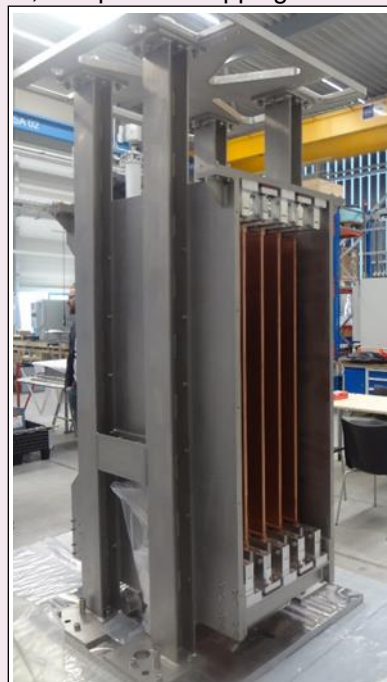
1 m long, 1.8 m high, 5 ton, Residual Ion Dump consisting of an assembly of 50 individual water cooled elements of CuCrZr to separate ionic component of the beam from the neutrals. Alternate panels of the assembly at high voltage and ground potentials.
