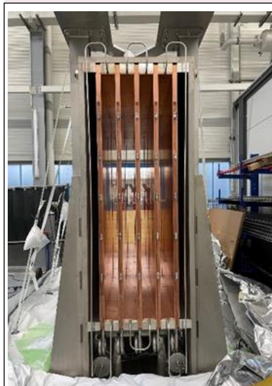
3 m long, 1.8 m high, 17 ton, 5 panel Neutraliser for DNB. Each panel is an assembly of consisting of 1 m long sub-panels made from CuOF. The panels are water cooled using a serpentine pattern of the deep drilled water channels in the horizontal and vertical direction. Extensive use of EBW is used to close the open channels in panels and for realising CuOF-Ni-SS transition for connecting the component to the cooling water system (view from downstream side)
