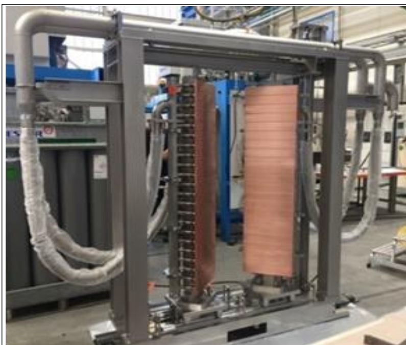
1.8 m high, 3 ton, 2 panel calorimeter assembly. Each panel is a stacked assembly of 22 HTE's made from CuCrZr. EBW has been extensively used to realise CuCrZr-CuCrZr and CuCrZr-Ni-SS joints of each HTE.
