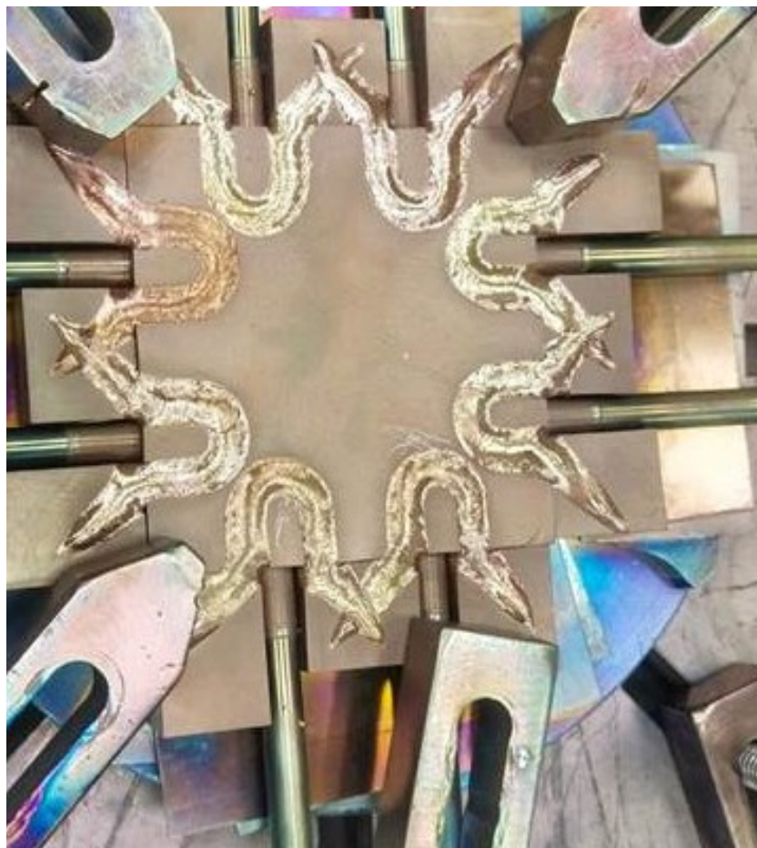
Welded PG prototype segment
