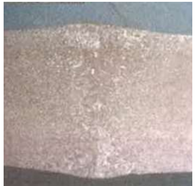
Micro examination of the weld joint (Cu-Cu)
