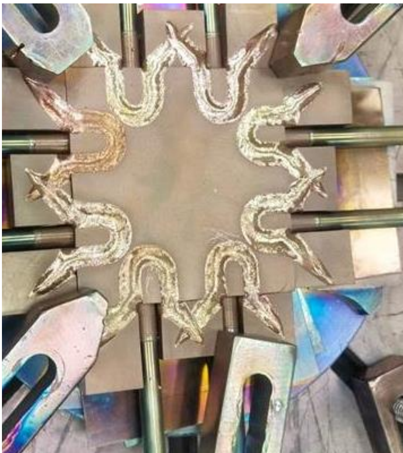
Welded PG prototype segment
